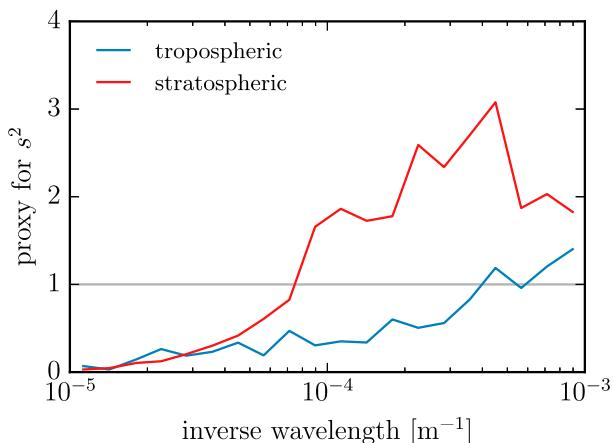
FIG. 6. Tropospheric ratio  $S^w(k)/S^b(k)$  and stratospheric ratio  $N_2^2 S^w(k)/N_1^2 S^b(k)$  as proxies for  $s^2 = \omega^2/N_1^2$  from the START08 data, assuming a monochromatic wave field.
